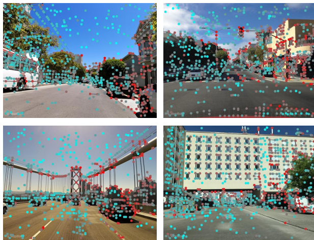
Fig. 3. Visualization of the attention weights computed by SuperGF on the input local features. Red dots indicate local features with high weights and cyan dots indicate those with low weights.
