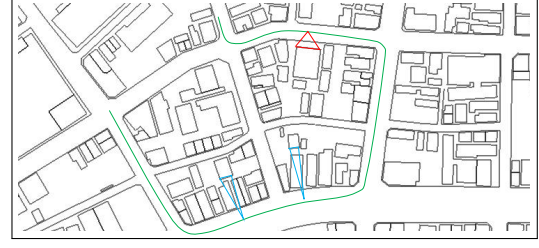
Figure 5. Illustration of differences in observation of individual buildings (best viewed in color). A building close to the camera trajectory (the green curve) will have a large viewing angle (the red triangle). A building can be occluded by others (the blue triangles). How a building is observed in the images determines the size of the point cloud emerged. Observe also that potential occlusion makes the building existences mutually dependent.
