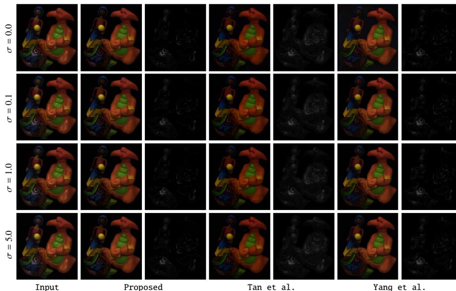
**Fig. 4.** Results for noisy input images. Zero-mean Gaussian noises with  $\sigma = 0.1, 1.0,$  and  $5.0$  are added to each pixel of each channel of the original image of the top row.
