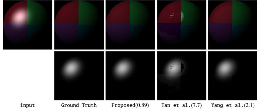
**Fig. 2.** Input image, ground truth, and separation results by the three methods. The numbers in the parentheses indicate the errors of the separated specular components.
