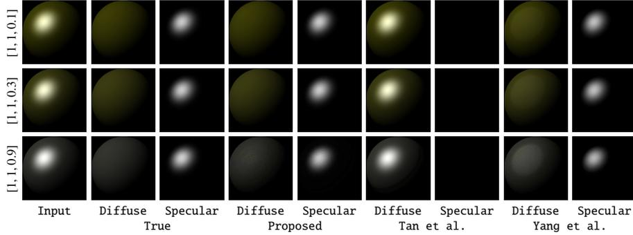
**Fig. 3.** The results when the body color is close to the illumination color. From top row to bottom,  $[R, G, B] = [1, 1, 0.1]$ ,  $[1, 1, 0.3]$ , and  $[1, 1, 0.9]$ .
